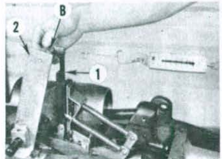
Fig. 222—Refer to text for testing and adjustment of draft control linkage.
