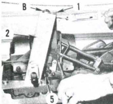
Fig. 224—Use a screwdriver to move pivot bracket while checking for correct setting. Refer to text.
