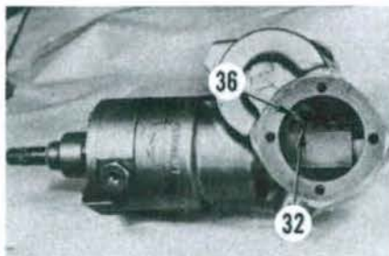
Fig. 16—The marked tooth of the left pinion (36) should be meshed with the center valley of rack (32).
